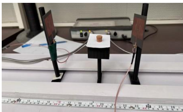
Figure 4.21: In experimental setup, cork model positioned at the center, 100 mm from each antenna, with a total separation of 200 mm between Antenna 1 and Antenna 2
