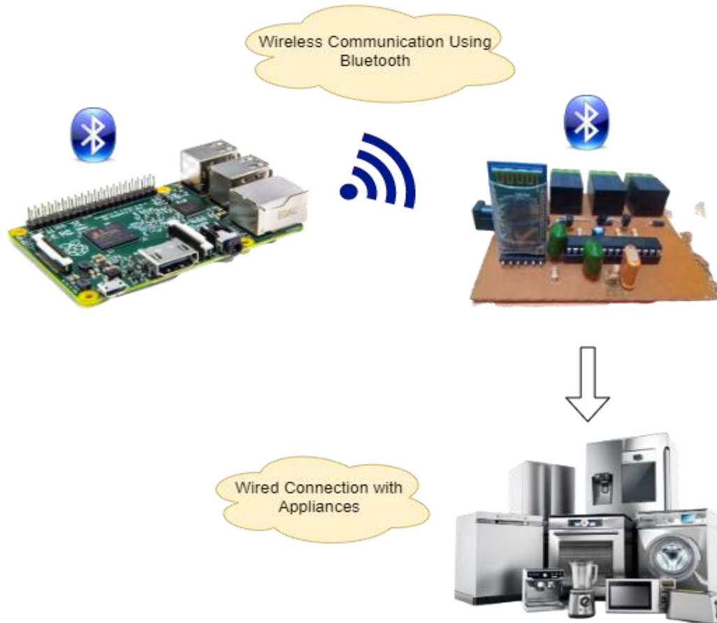
Figure 31. Relay with Appliances
