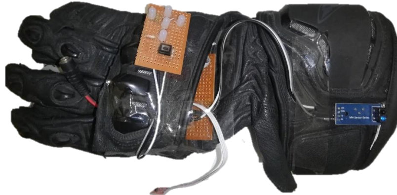
Figure 7: Bicycle gloves with module
