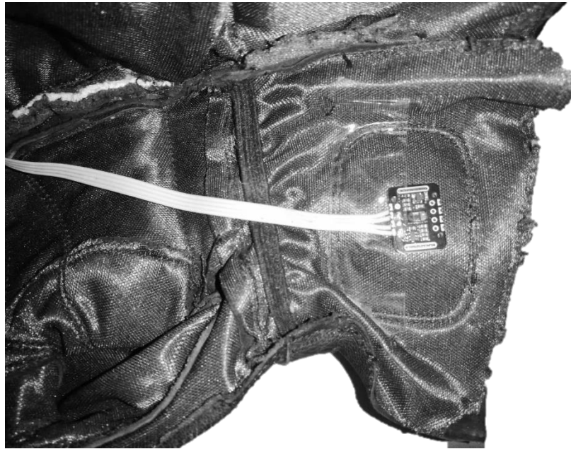
Figure 6: Touch sensor mounted on gloves with stitched pockets
