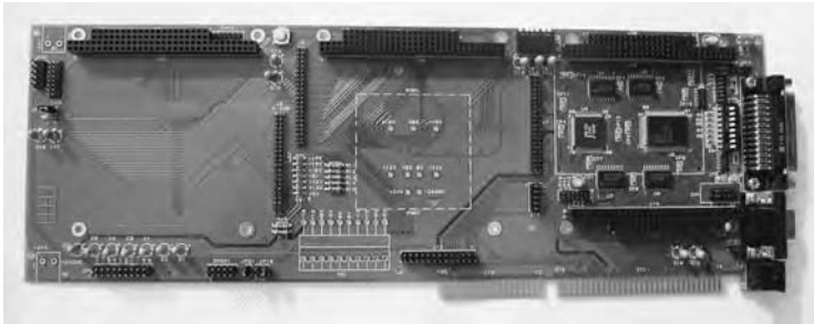
Figure 5.6 Slave board without modules (the dual RAM is visible on the left side)
