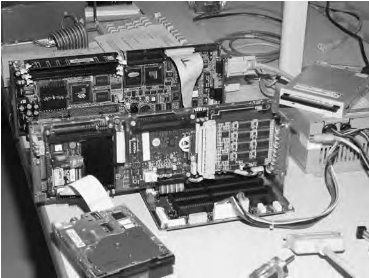
Figure 5.4 Photograph of the passive bus equipped with a master card and a slave card
