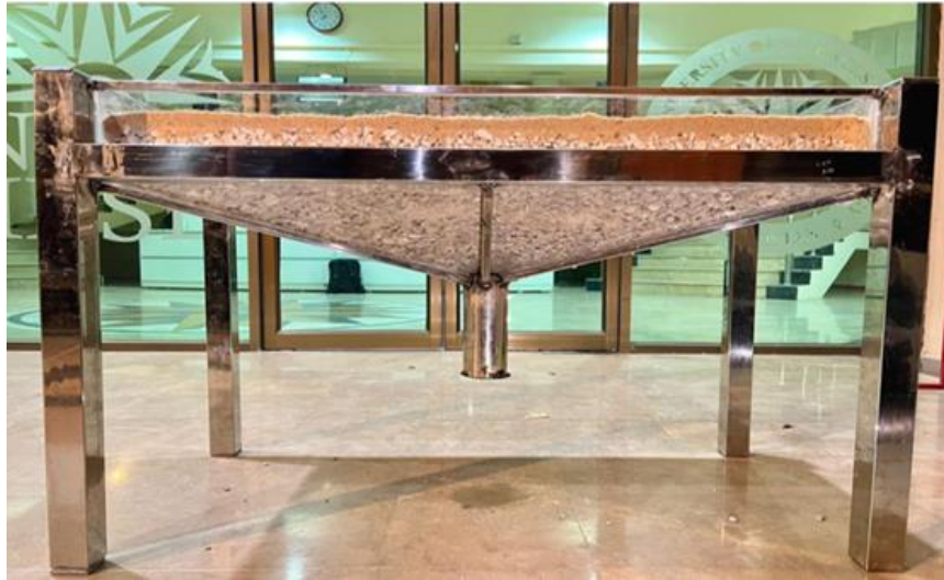
Figure 4.5 shows the fabricated lab-scale sludge drying bed.
