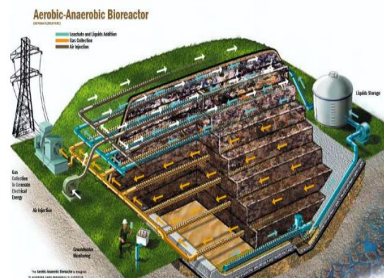
Figure 9 Aerobic-Anaerobic bioreactor landfill
