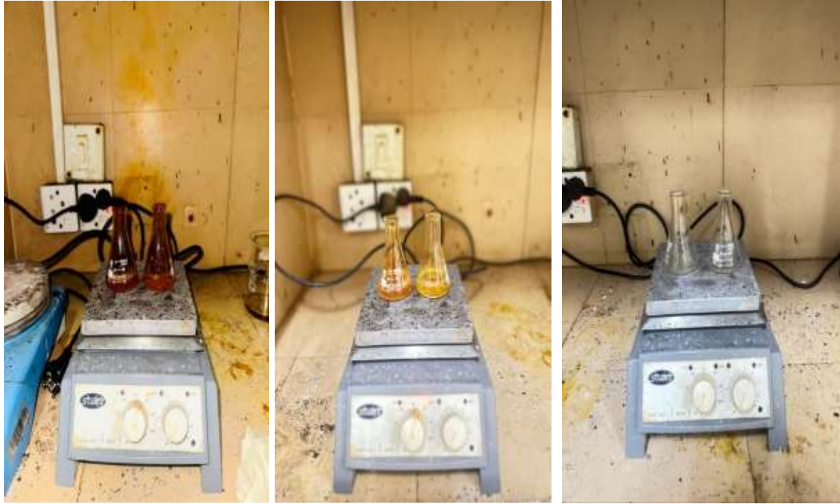
Figure 7: (a): Sample preparation for AAS analysis through wet digestion method
