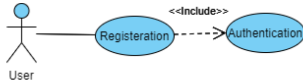
Figure 2.5 Usecase Diagram for Registration to the application. The user is required to enter a username and password which is authenticated by the database. After Registration, the database tables are updated accordingly.
