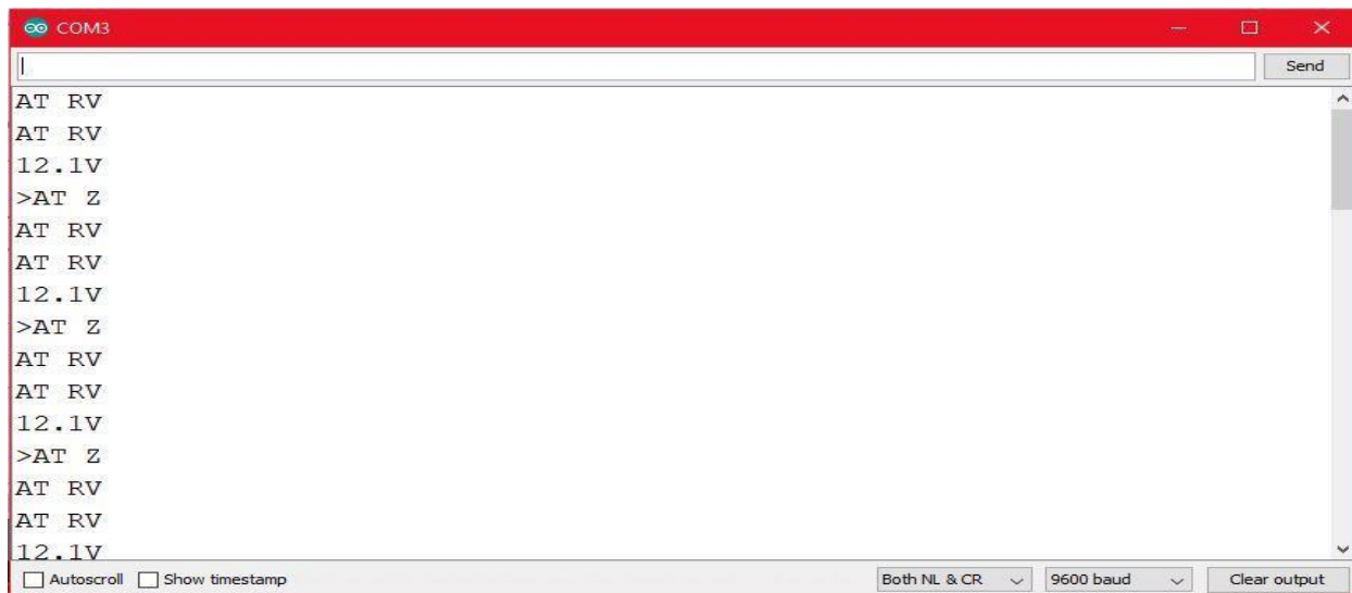
Figure 24: Battery Voltage Results
