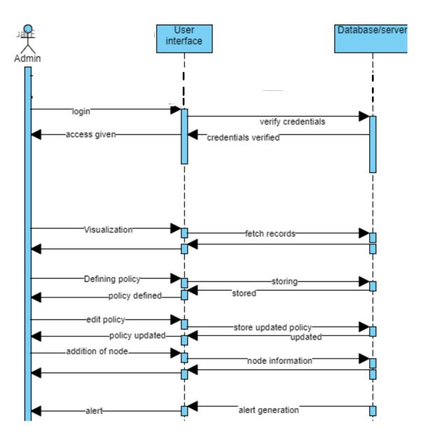
This is the sequence diagram of the system in which admin logs in to the system if credentials are right access is given to him then on the dashboard there are multiple options available where he can visualize the network traffic, define policy, edit it add node to the network and generate alerts.
