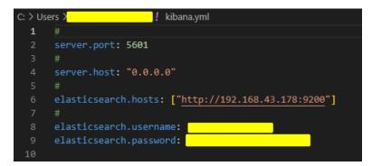
This is the Kibana module configuration mentioning that Kibana runs on localhost port 5601 and is accessible from within the network conditioned with credentials. The Kibana visualizer gets its input data from the Elasticsearch server.
