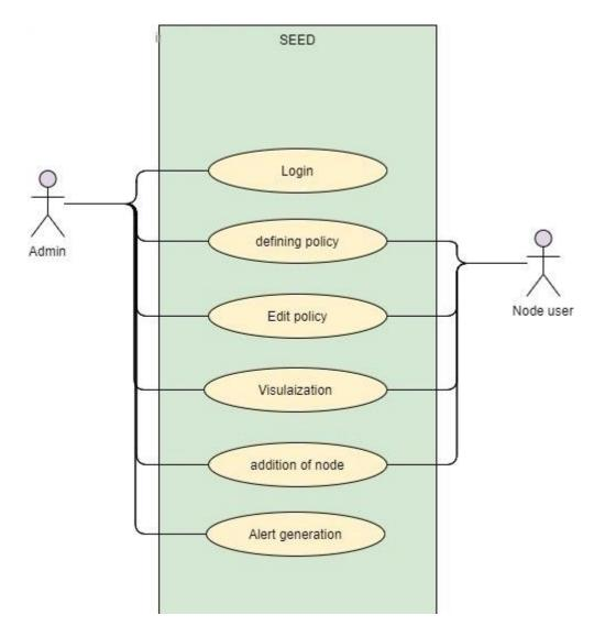
This is the use case diagram of the in which admin and the node user have interactions. The admin can login by entering his credential define policy edit it and can visualize the traffic. He can add another computer to the network which is addition of node by clicking on It and can generates alert.
