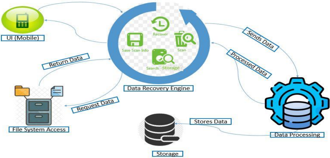
Figure 4: Architecture Diagram of Android Data Recovery Tool
