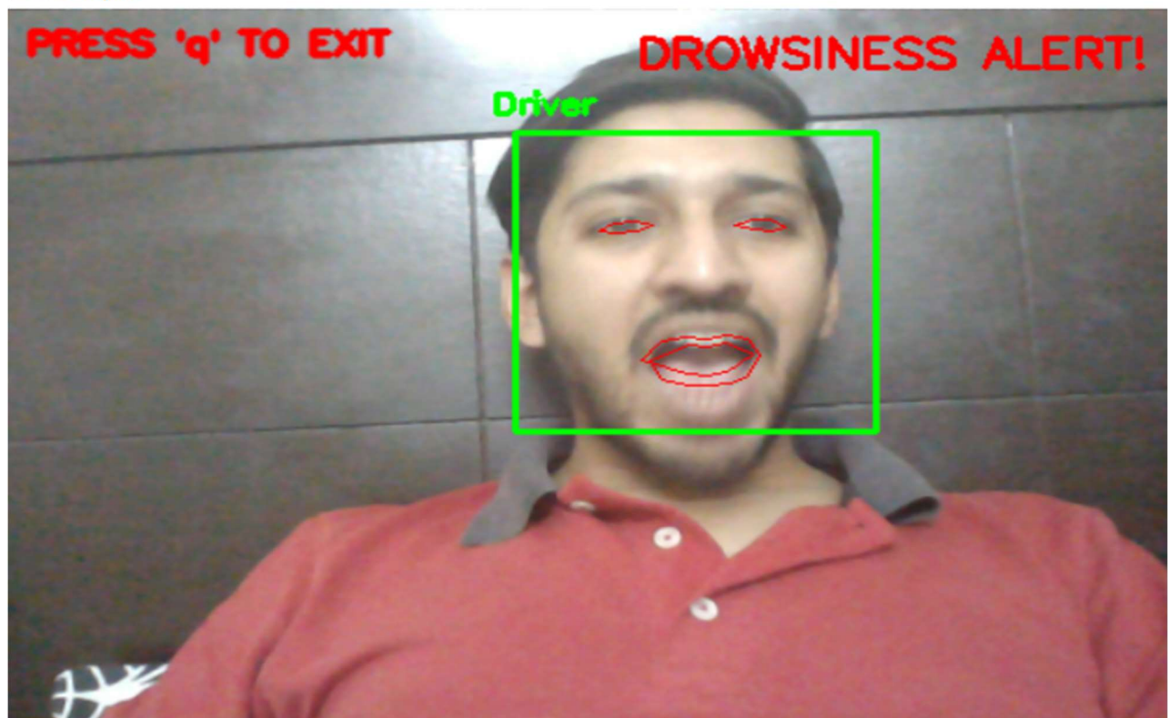
Figure 9: Detection of Yawning, It Shows Driver is Drowsy
