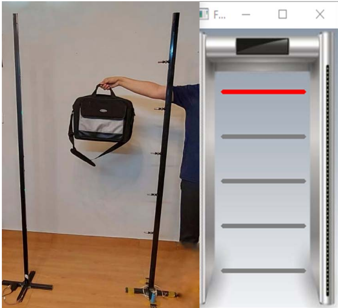
Figure 12. When a bag distorts the laser beams.
