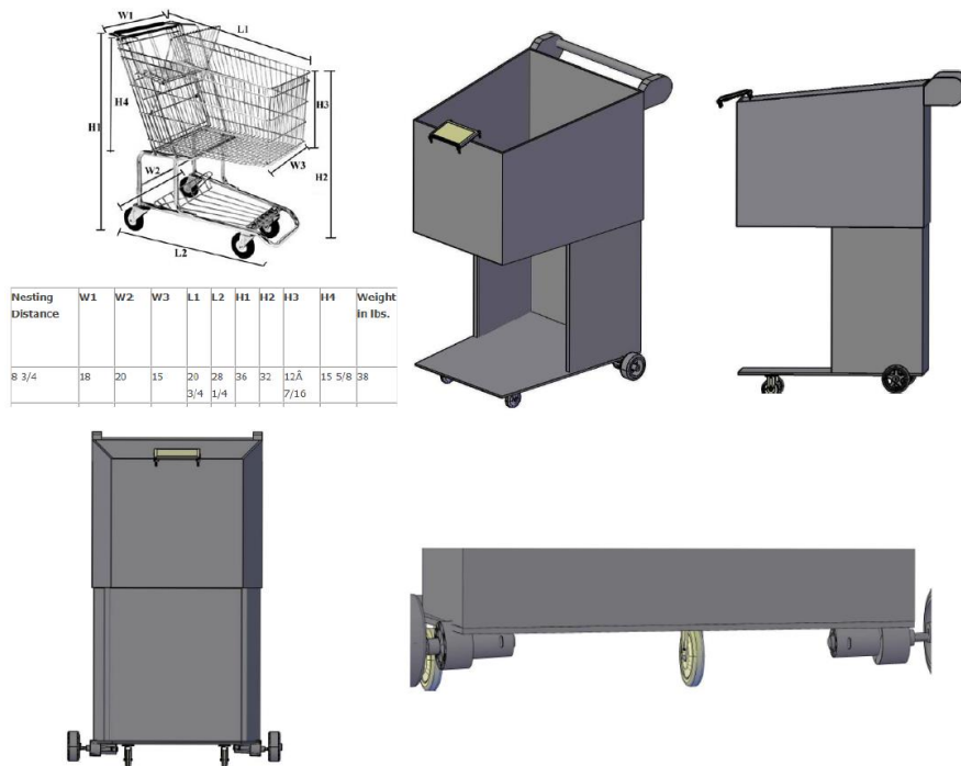
Figure 2: AUTOCAD created Chassis design
