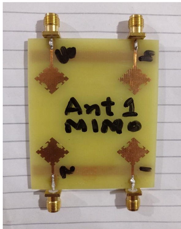
Figure 3.11: Top View of 4-element dual band MIMO after fabrication and soldering of connectors
