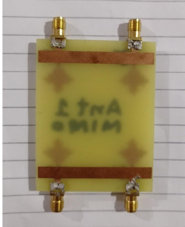
Figure 3.12: Bottom View of 4-element dual band MIMO after fabrication and soldering of connectors
