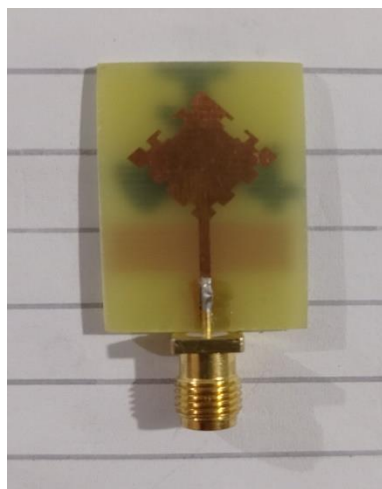
Figure 3.7: Top View of Single element dual band after fabrication and soldering of connectors
