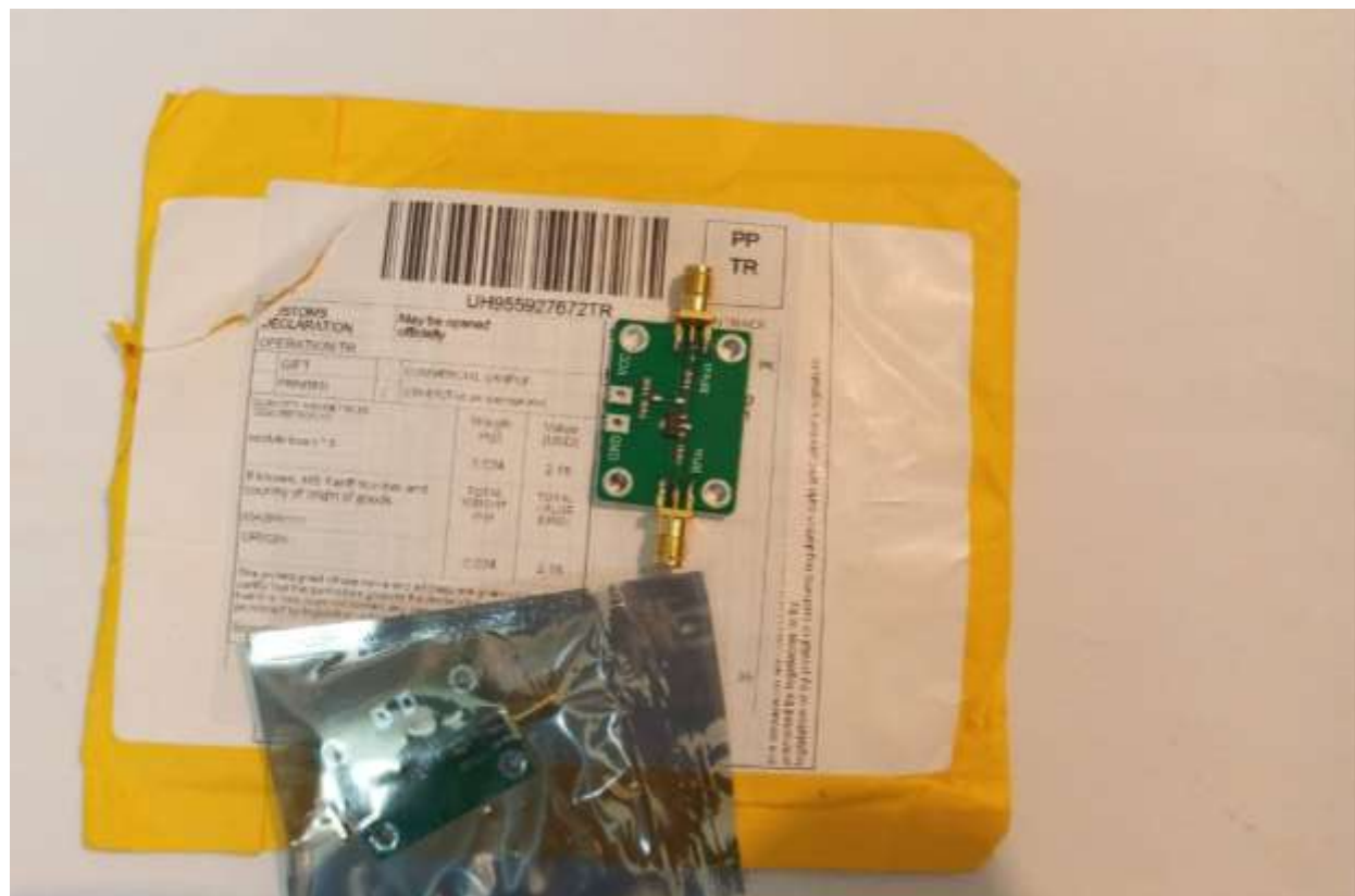
Figure 4.12: TQP3M9009 LNA module used
