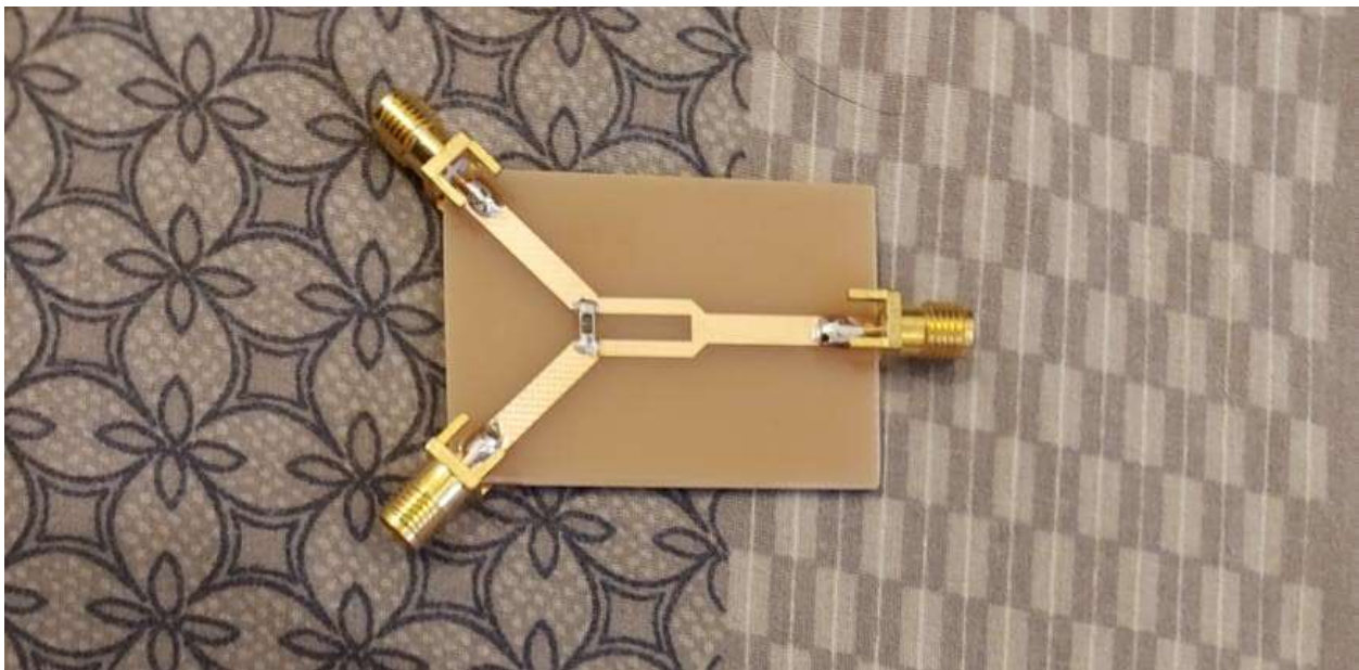
Figure 3.12: Fabricated single Wilkinson Power Divider
