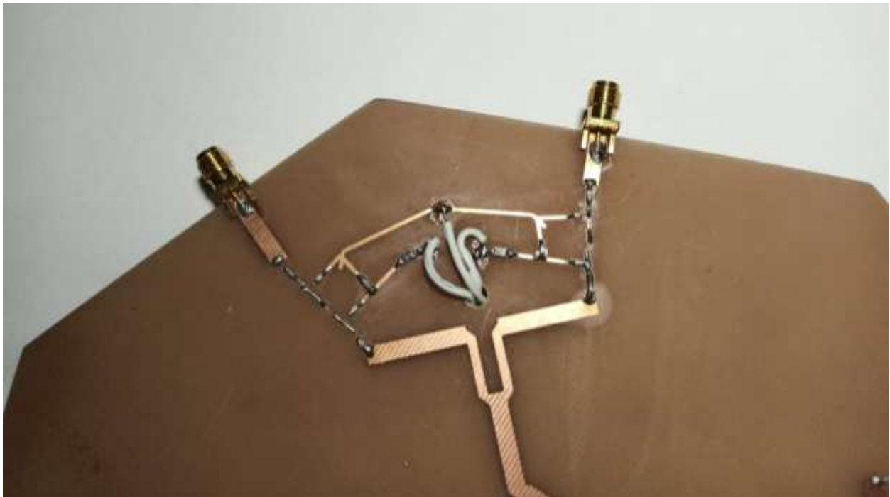
Figure 5.20: PiN Diode Switching Network assembly with SMD components soldered and wires for VCC and Gnd input added
