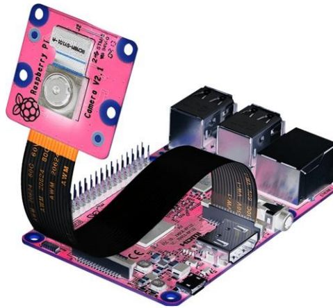
Figure 4.1: Alternative Approach using Pi Camera with Raspberry Pi
