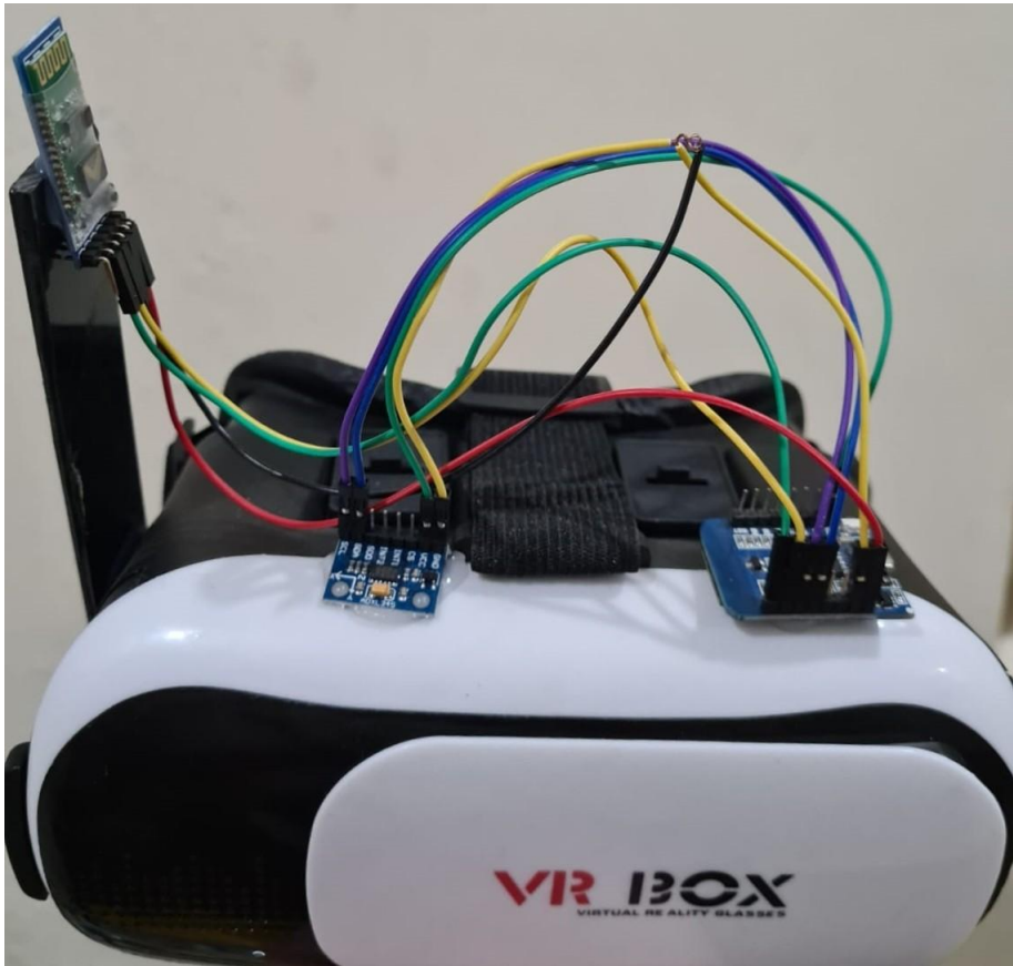
Figure 6.6: Complete connection of VR Headset with different modules
