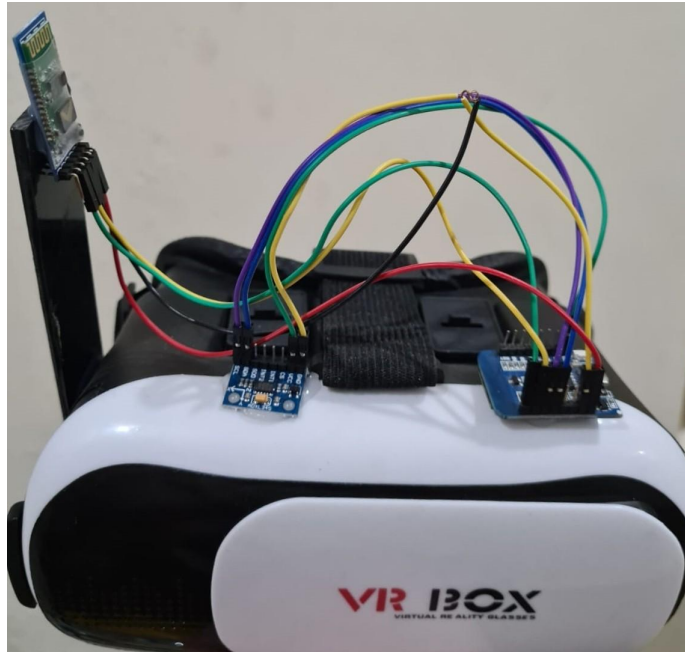
Figure 5.5: Accelerometer Sensor, ESP8266 and Bluetooth Module at-tached to VR Headset
