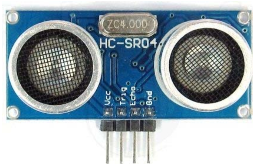
Fig. 3. 2: HC-SR04 ultrasonic sensor
