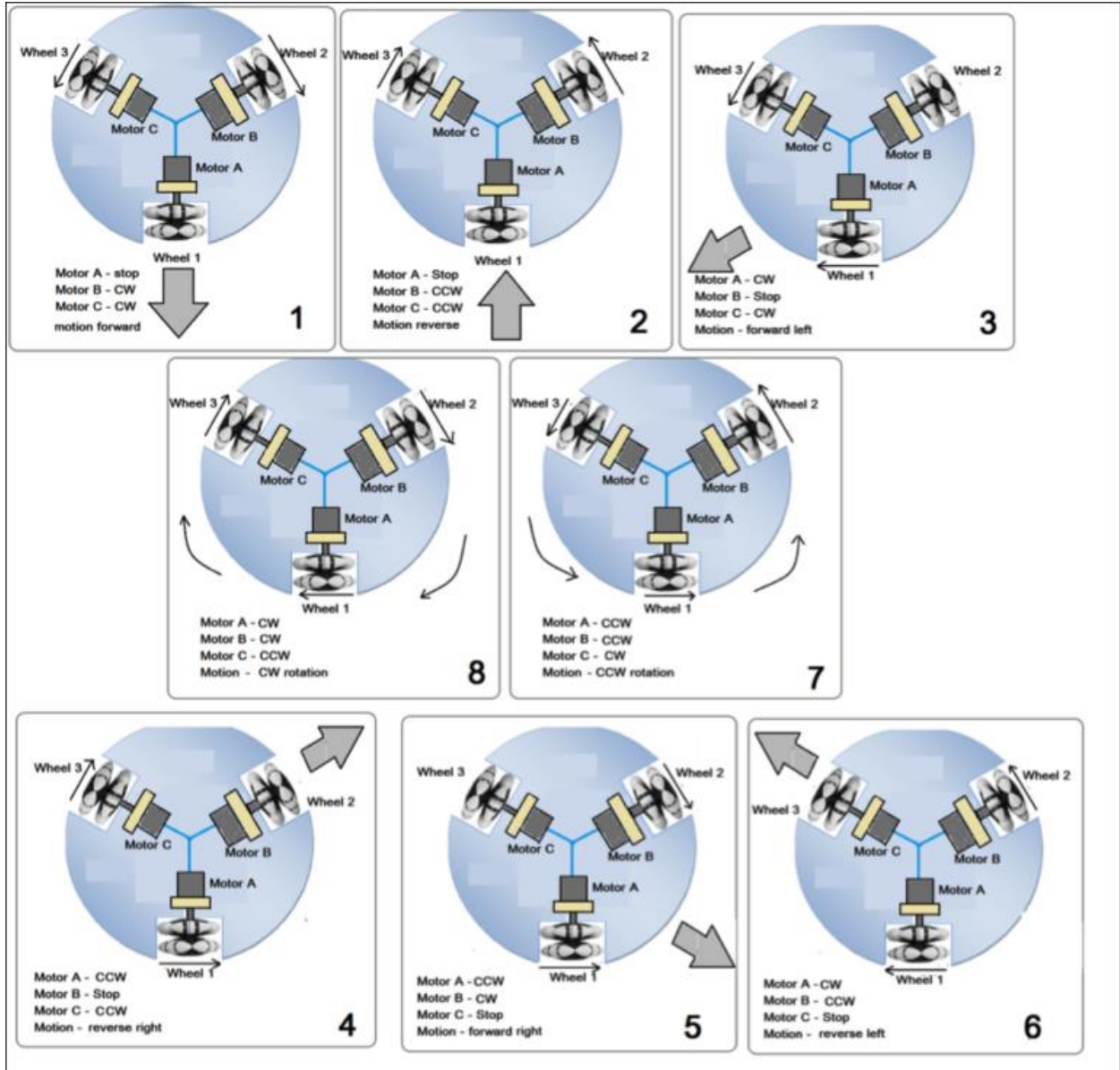
Fig 18: Movement of Robot in different directions [28]
