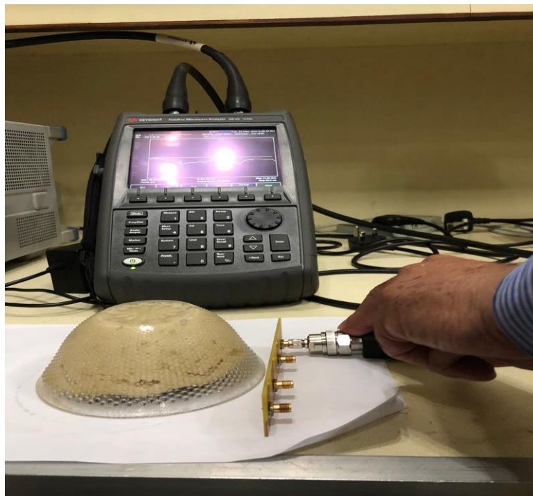
Figure 5.1 Real Time Measurement of S_{11} using VNA
