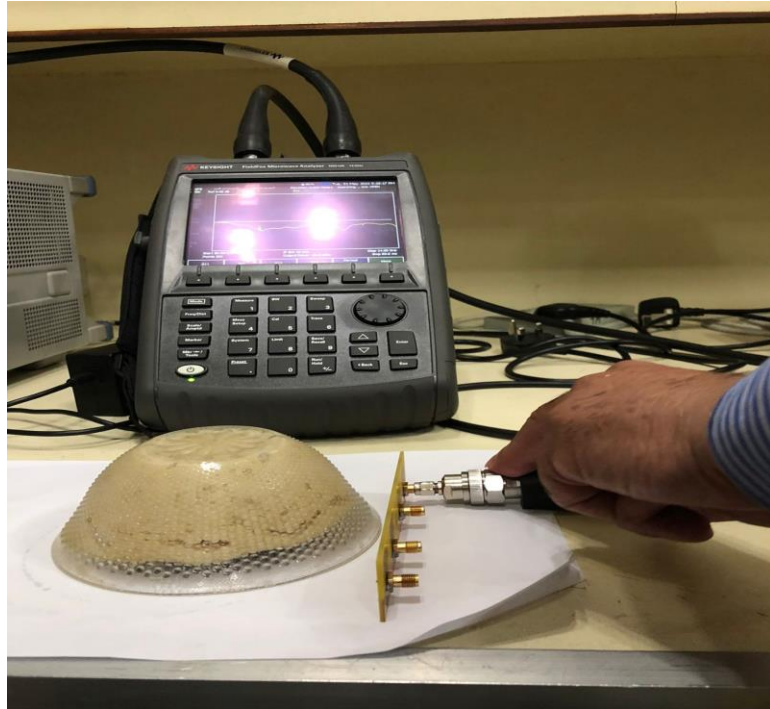
Figure 57: Real Time Measurement of S_{11} using VNA
