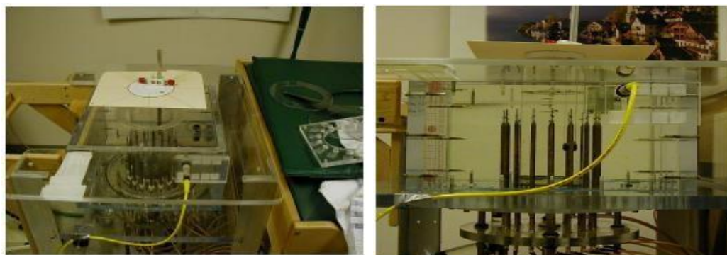
Figure 3-4: The Dartmouth College microwave imaging system. [10]
