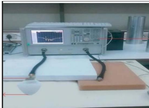
Figure 5-1 Experimentally measuring S_{11} Signals
