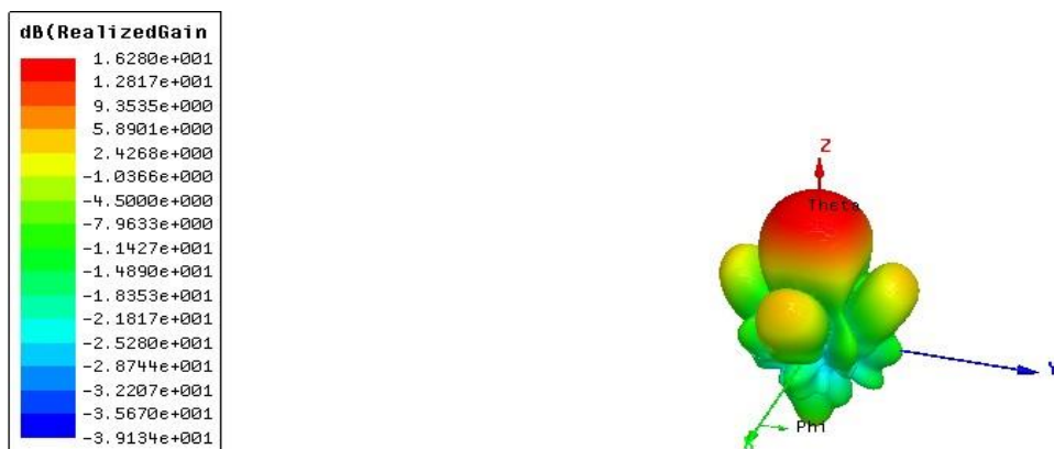
Figure 4.6: Gain of 4x4 is 16.28 dB
