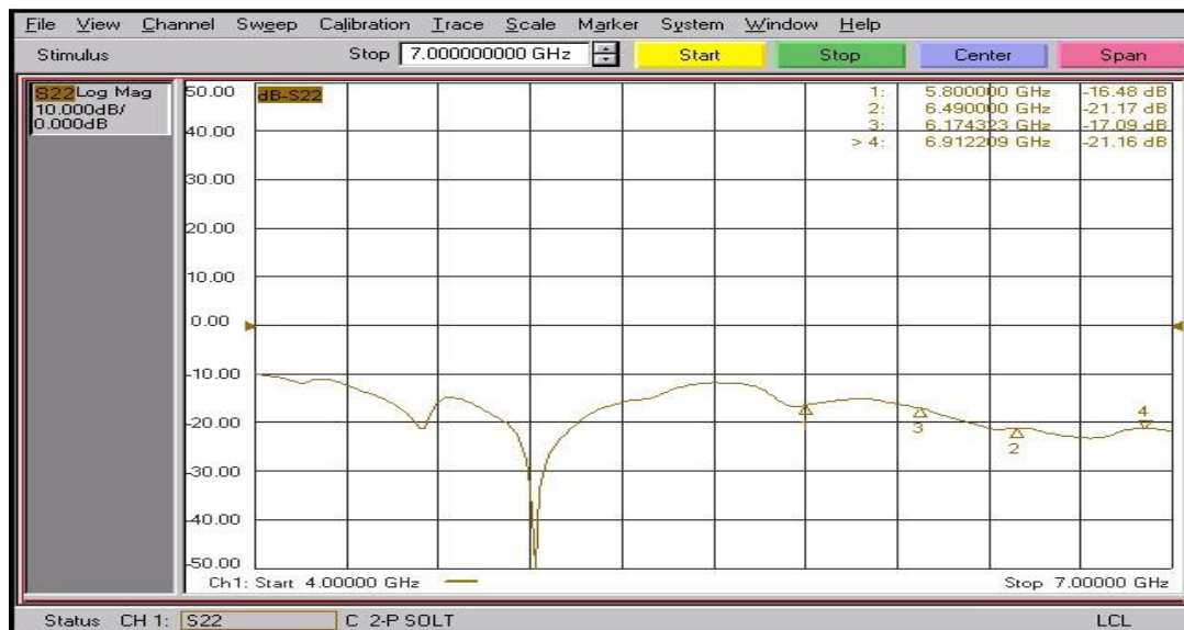
Figure 4.12: practical results of matching port
