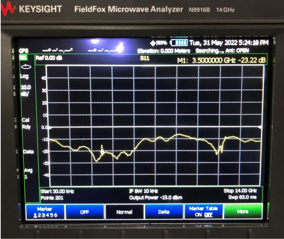
Figure 4.1: S11 at 3.5 GHz is -23.22 dB
