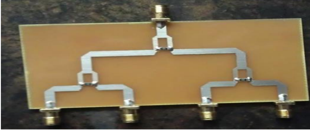
Figure 5.12: Design of power divider in ADS
