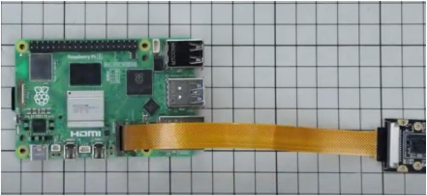
Figure 7. Pi Camera Module V1.3 Connections
