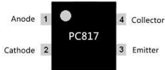
Figure 7: Optocoupler Pin Configuration
