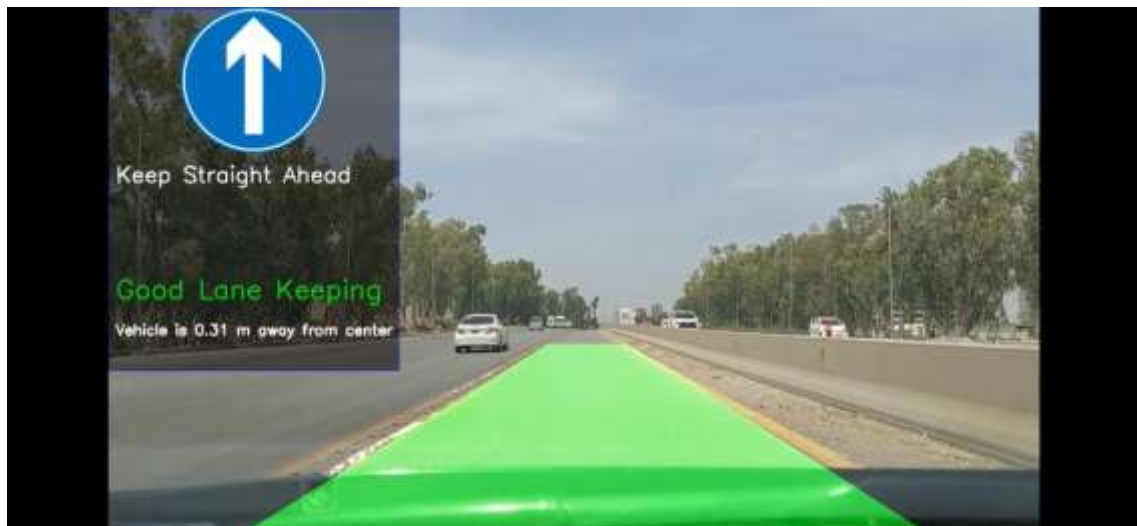
Figure 5.6 Navigation of straight line on the road
