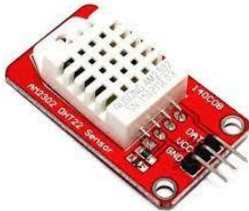
Figure 3 DHT-22 Temp/Humidity Sensor
