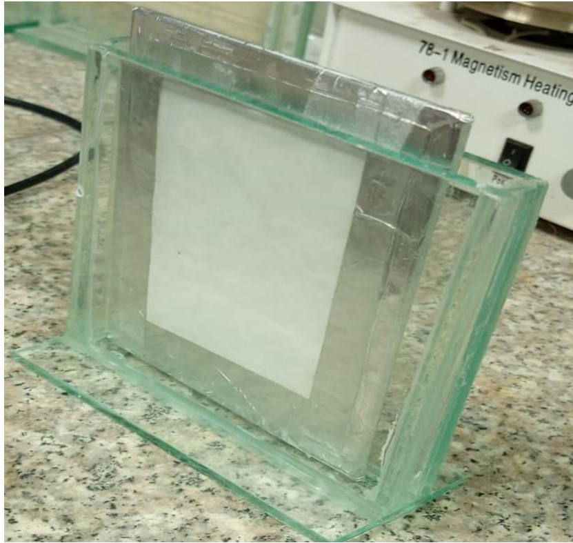
Figure 5: Pretreatment in DI water before TFC casting
