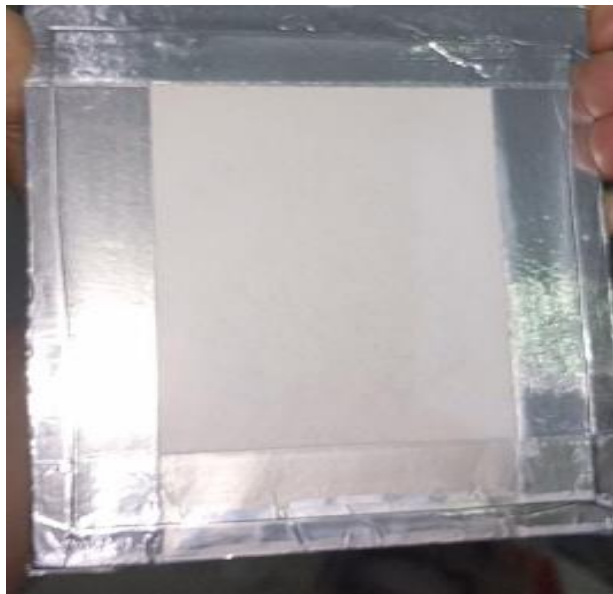
Figure 4: PSF Sheet wrapped in Aluminum Tape
