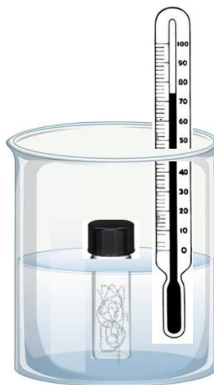
Figure 3.3: Setup for synthesis of one-step shape memory polyurethane
