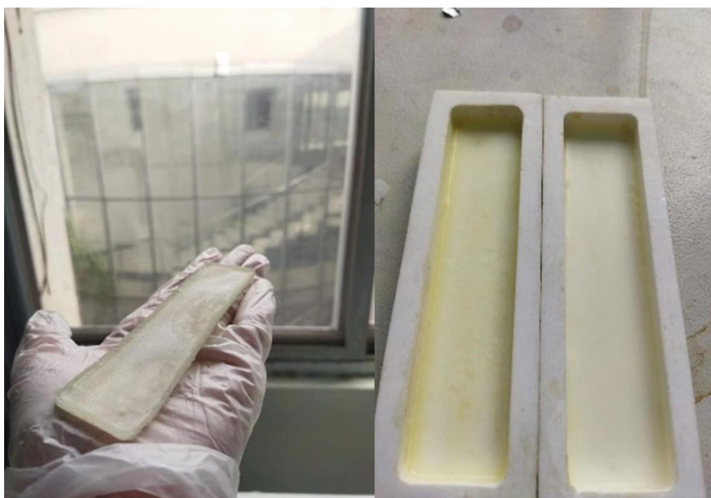
Figure 3.5: Teflon mold and synthesis of free-standing shape memory polyurethane films
