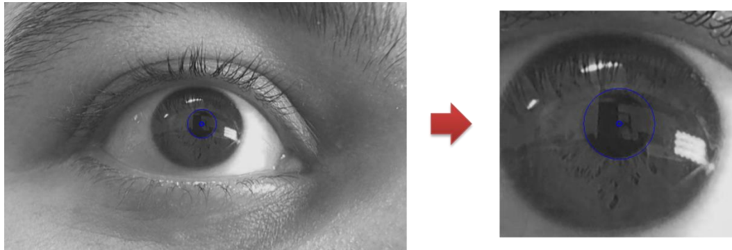
Figure 10: Detected pupil region and fitted ellipse through Hough ellipse transform
