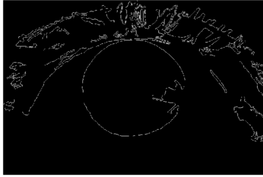
Figure 6: Edge map obtained after applying Canny edge detector and thresholding
