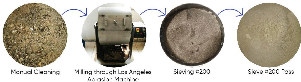
Figure 3.3: Preparation methodology of MIBA for study
