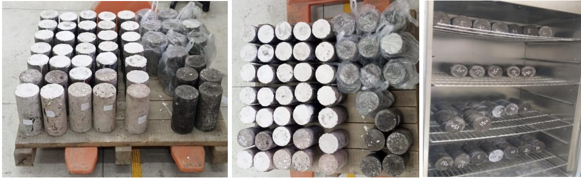
Figure 3.6: Casted sample and their heated curing in oven
