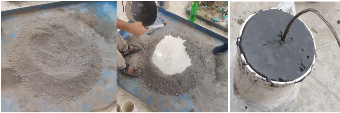
Figure 3.5: (a) Mixing and casting of AAC sample (b) sample with a thermocouple for temperature measure during elevated temperatures
