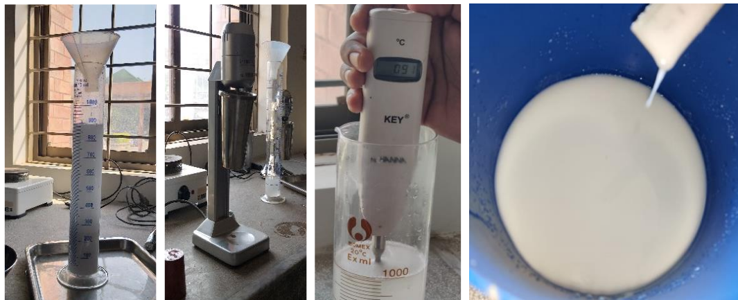
Figure 3.2: Preparation of Alkaline activator solution
