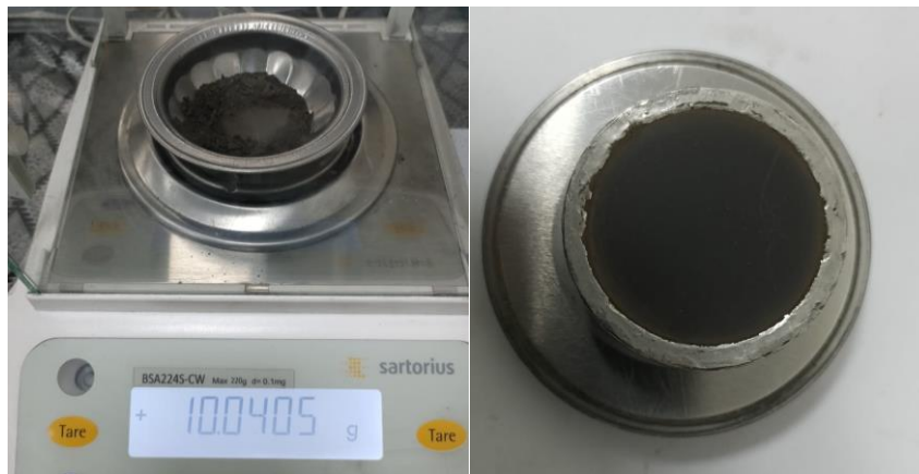
Figure 3.4: MIBA sample preparation for XRF analysis
