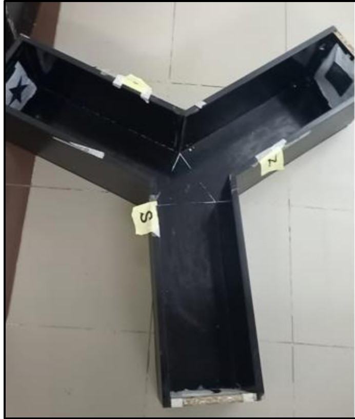
Figure 2.5: Y-maze apparatus used for behavioral testing. The figure depicts the Y-shaped maze designed to assess spatial memory and exploratory behavior in mice. The three identical arms are arranged at 120° angles, allowing for the evaluation of spontaneous alternation performance.
