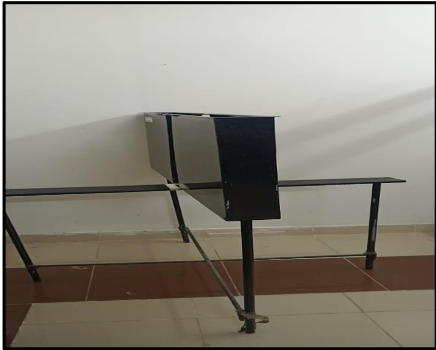
Figure 2.6: Elevated Plus Maze (EPM) set up for anxiety-like behavior assessment. The figure depicts the plus-shaped apparatus elevated above the ground, consisting of two open arms and two enclosed arms. The setup is used to evaluate exploratory behavior and anxiety levels in mice, based on their preference for open versus enclosed arms.
