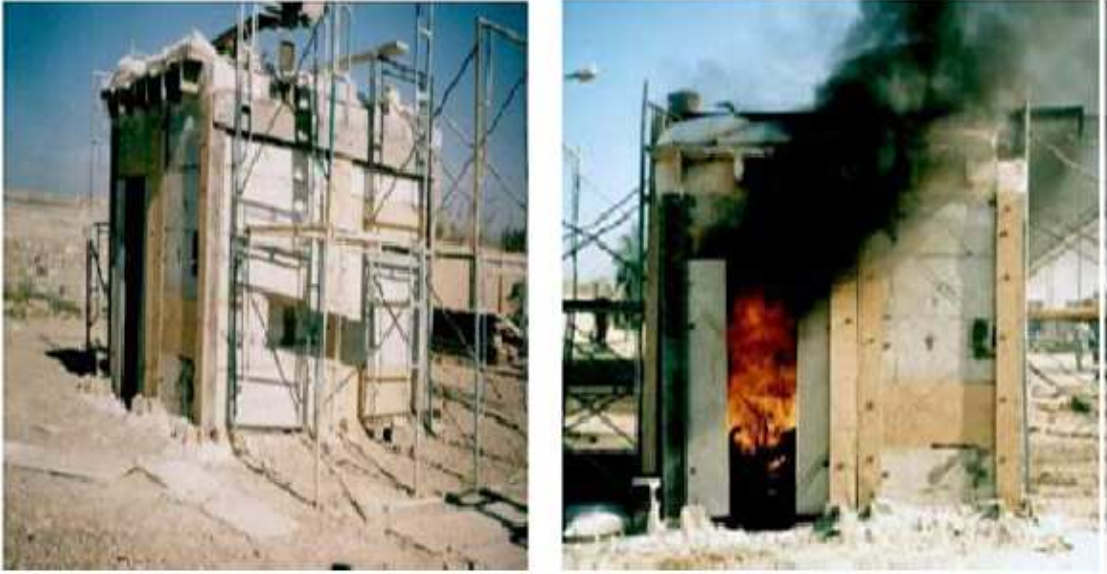
Fig 5.2: Fire Resistance tests on ferrocement buildings at Ferrocement Factory, Baghdad, Iraq.
