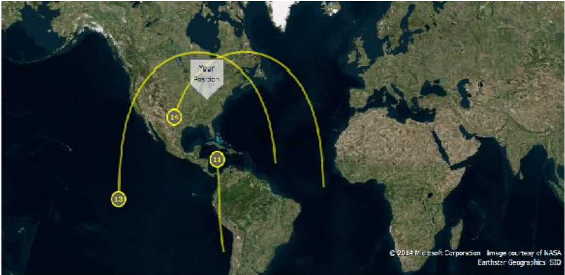
Fig 6.15 Tracks of Beidou-2 Satellites over Ohio State
