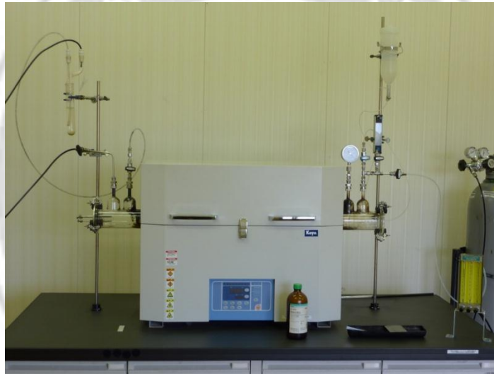
Fig.2.8 Chemical vapor deposition method
