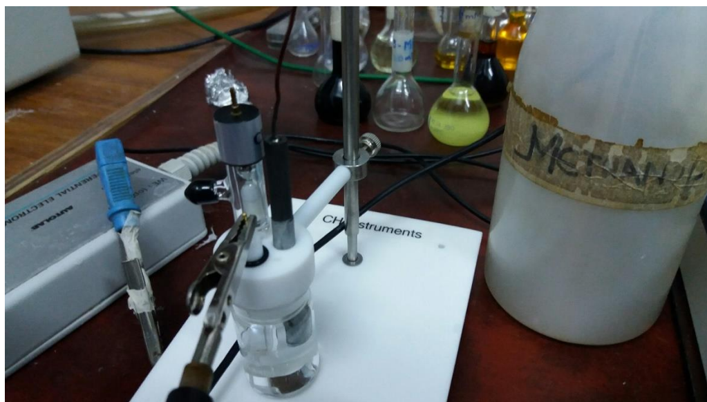
Figure 4.4 Conventional three electrode Pyrex glass cell
