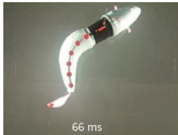
Figure 5. Fish t = 66 ms. The pressurizing of the tail causes it to deform with a curvature and produce a force.
