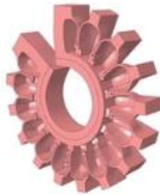
Figure 7. A Pneumatic Network (PneuNet) actuator.
