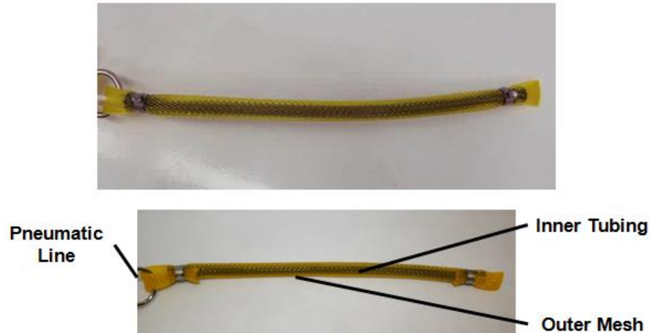
Figure 6. A diagram of the structure of a pneumatic artificial muscle.
