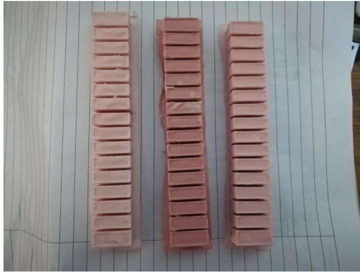
Figure 33. Fabricated PneuNets actuators.
