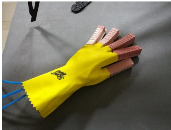
Figure 34. Completed soft prosthetic hand.
