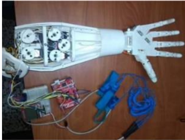
Figure 2. A full disassembled picture of a modern prosthetic hand showing the number of bulky parts involved, depicting a lack of human-friendly design.
