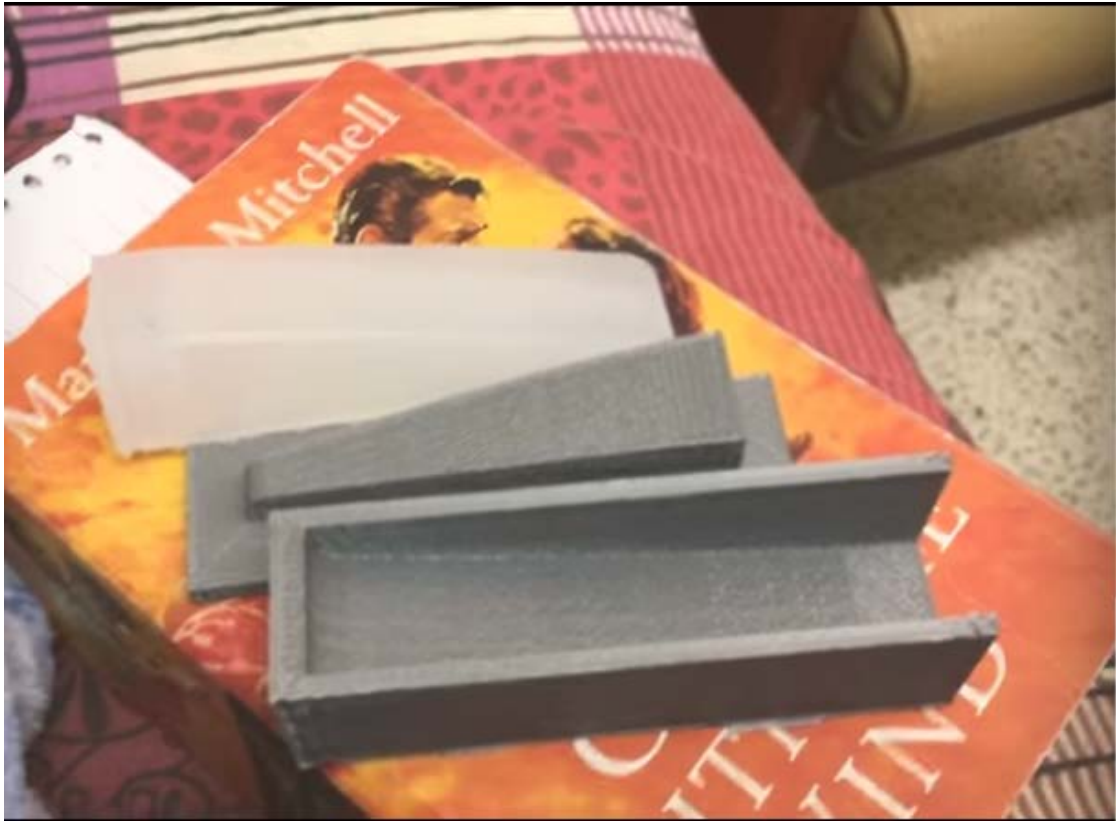
Fig. 16 (Our mold and a sample silicone casting)
