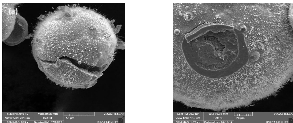
Figure 9. CuO nanowires with an oxidation time of 4 hours
