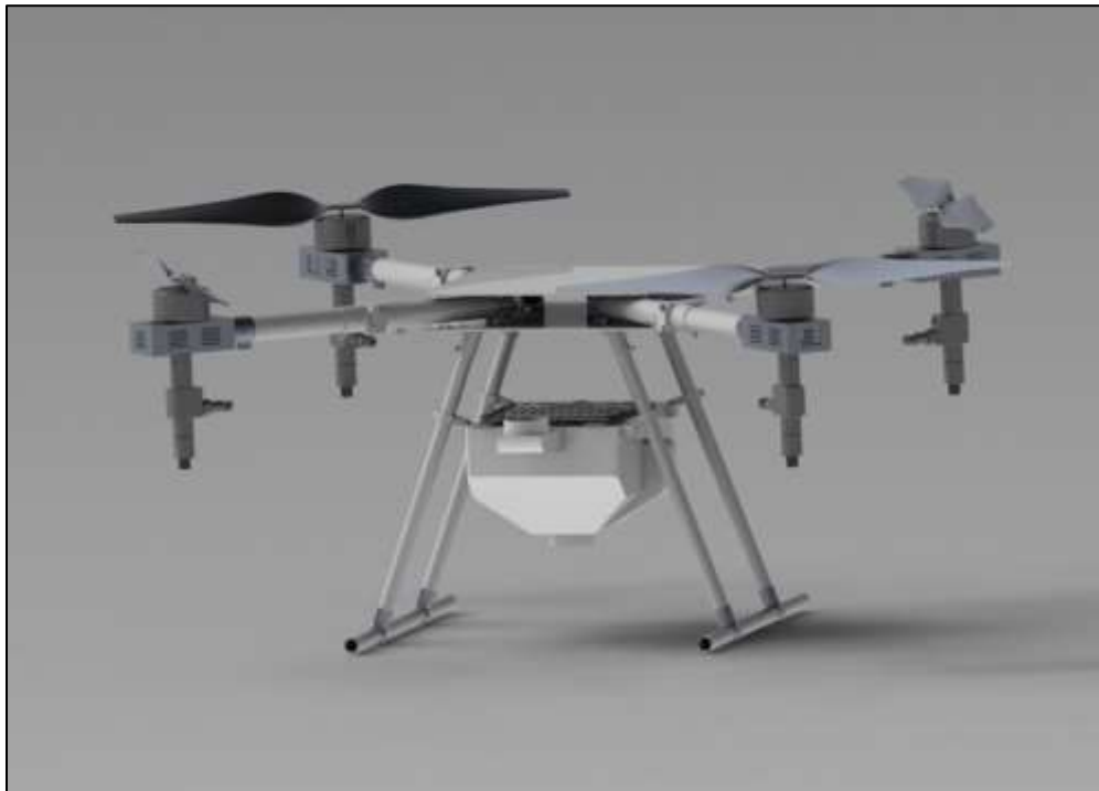
Figure 13: CAD model of complete drone with spraying system
