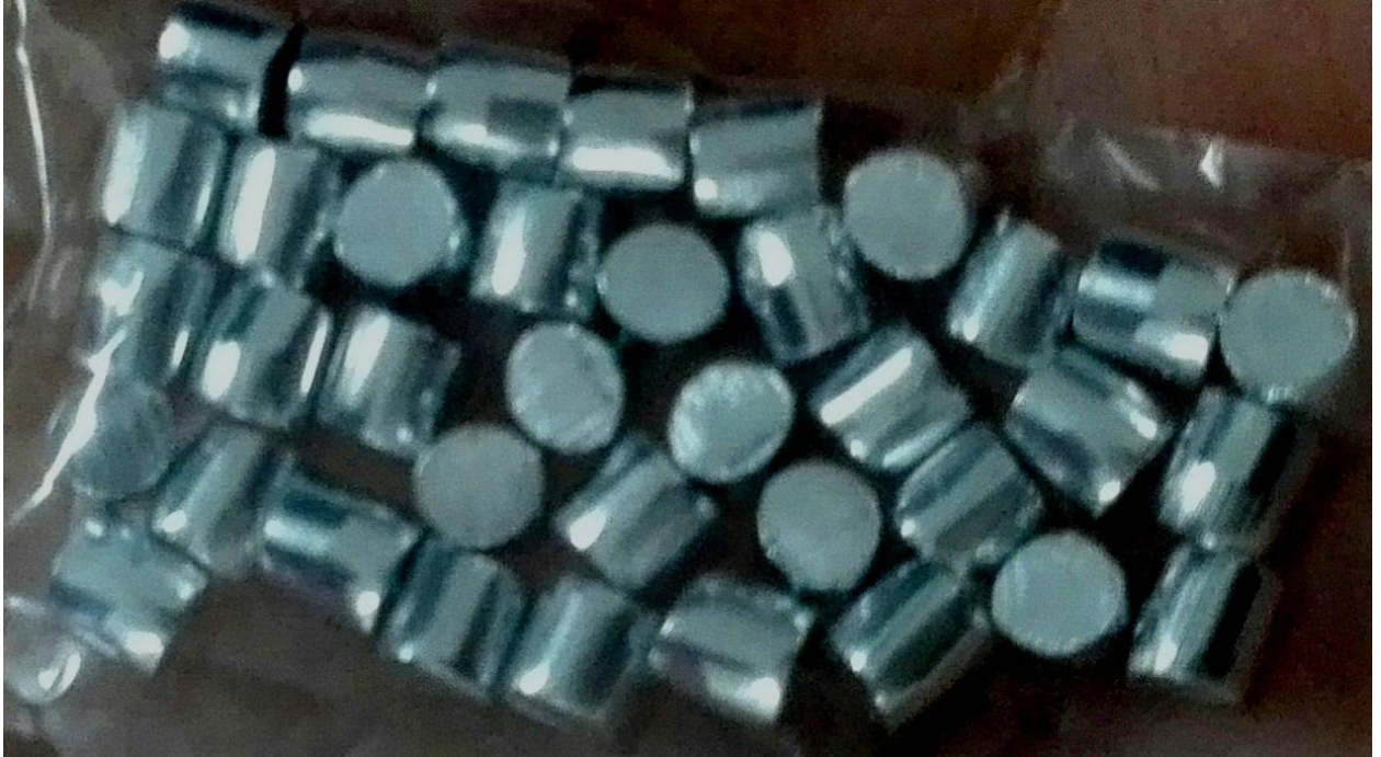
Figure 22: Cr Pellets (99.999% pure) Used in Thermal Evaporation
