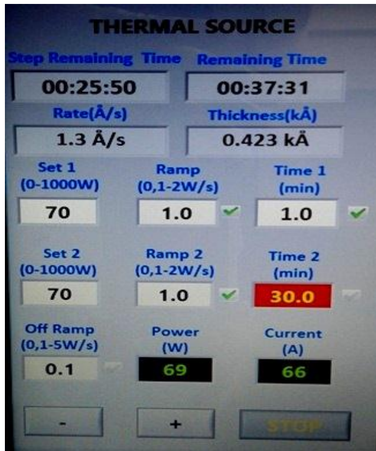
Figure 24: Parameters for Thermal Evaporation of the Al
