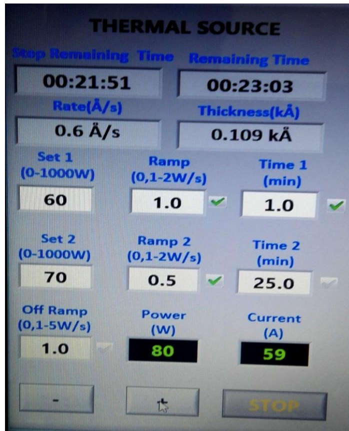
Figure 25: Parameters for Thermal Evaporation of the Ag
