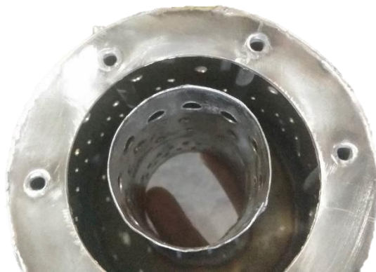
Figure 26: Fabricated Combustion Chamber
