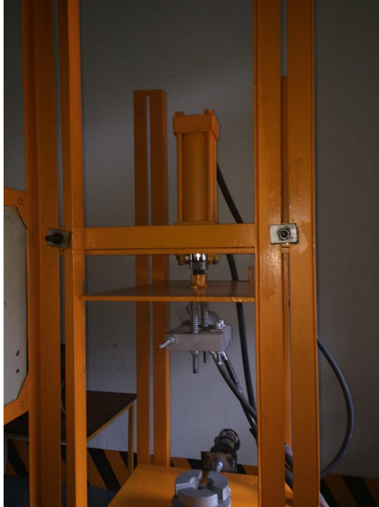
Figure 2.4: Motorized Clamping and Hydraulically actuated Pulling Action
