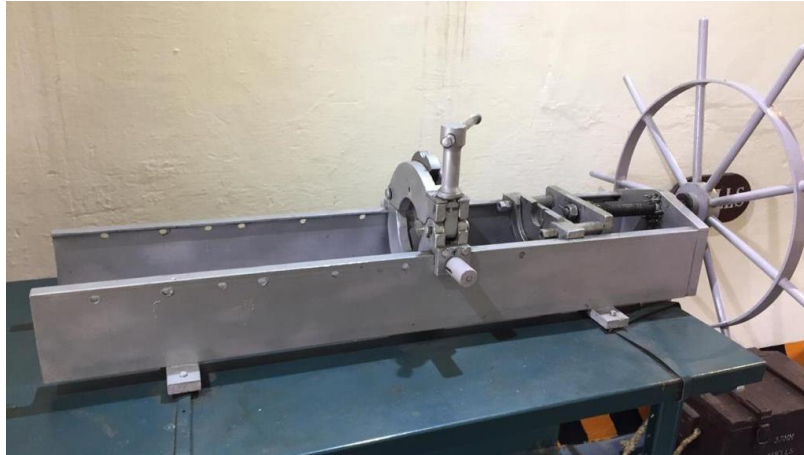
Figure 2.3: Manual Clamping and Manual Pulling Action
