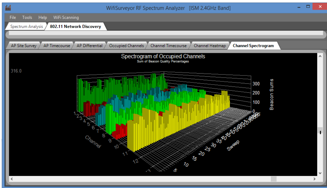
Figure 4.5: Channels Spectrogram by Deploying OSSA
