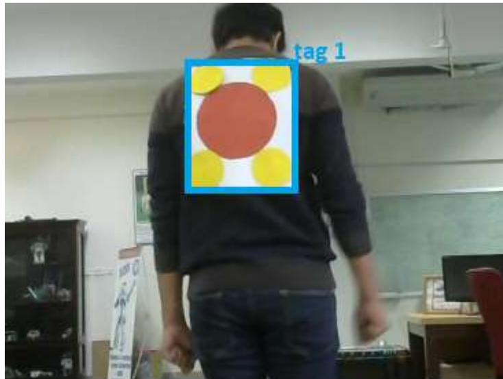
Fig. Tag detected and labelled by computer vision
