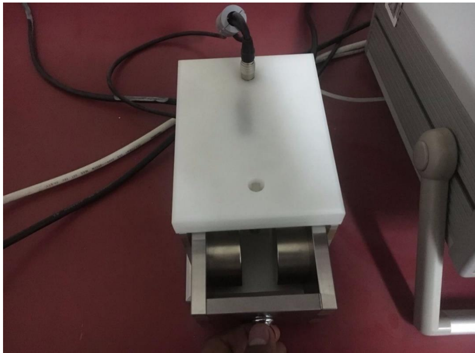
Figure 31: Sample kit with 0.55 Tesla magnet supplied standard with the system
