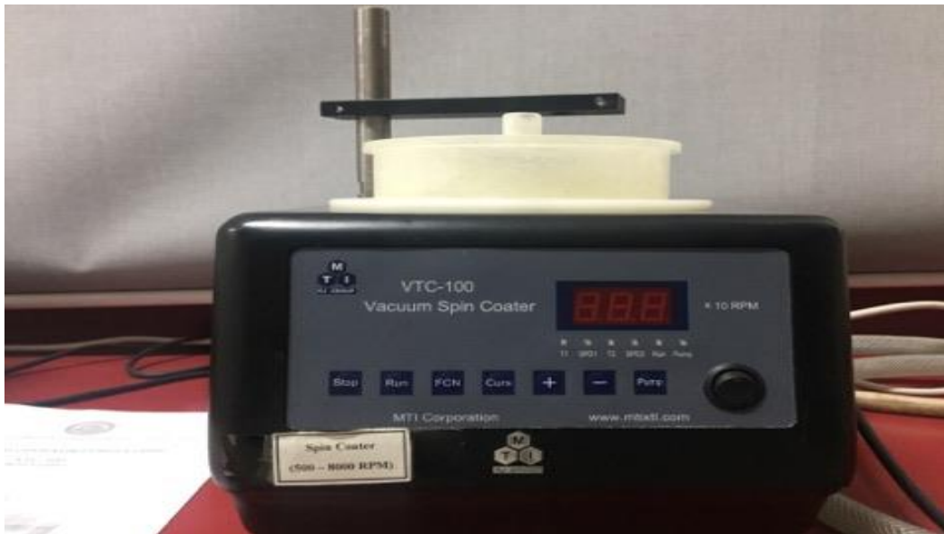
Figure 20: Spin coater in energy materials lab at USPCASE NUST
