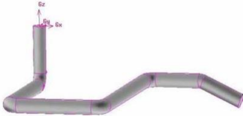
Figure 25 Pressurizer surge line model of CHASNUPP II [23]
