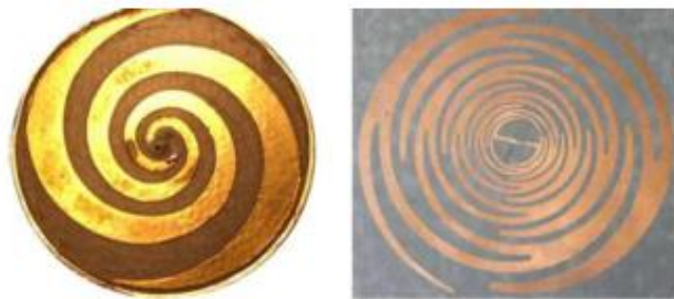
Figure 2.3 Printed Spiral Antenna [15]
