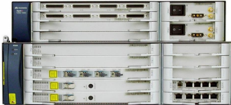
Figure 21 : NTC Switching system
