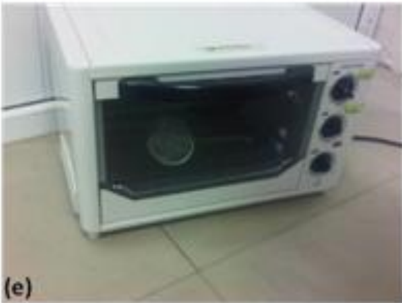
Figure 13. Acid pickling process of Coronary stents, (a) Acid pickling solution preparation, (b) Stents in ultrasonic cleaner, (c) stents rinsed in the sieve, (d) Stents after rinsing with propanol, (e) Sieve having stents is placed into an oven, (f) Acid pickled stents in Petri dish.
