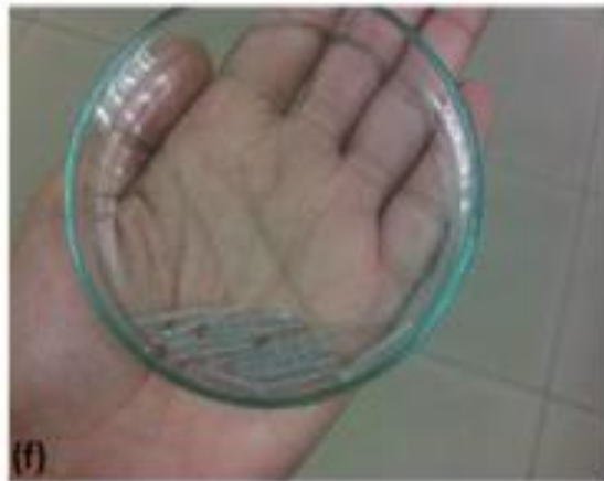
Figure 13. Acid pickling process of Coronary stents, (a) Acid pickling solution preparation, (b) Stents in ultrasonic cleaner, (c) stents rinsed in the sieve, (d) Stents after rinsing with propanol, (e) Sieve having stents is placed into an oven, (f) Acid pickled stents in Petri dish.
